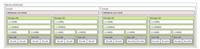
Developers using the hwloc API or XML output for portable applications should therefore be extremely careful to not make any assumptions about the structure of data that is returned. For example, per the above reported PPC topology, it is not safe to assume that PUs will always be descendants of cores.
