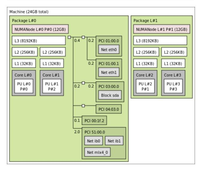
Six interesting PCI devices were discovered. However, hwloc found some corresponding software devices (*eth0*, *eth1*, *sda*, *mlx4\_0*, *ib0*, and *ib1*) for only four of these physical devices. The other ones (*PCI 102b:0532* and *PCI 8086:3a20*) are an unused IDE controller (no disk attached) and a graphic card (no corresponding software device reported to the user by the operating system).
