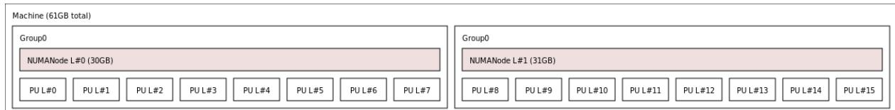
And here's the graphical output from lstopo on this platform when SMT is disabled:
