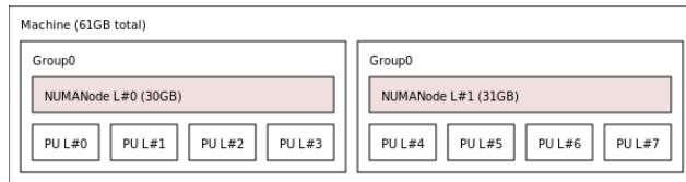
Notice that hwloc only sees half the PUs when SMT is disabled. PU L#6, for example, seems to change location from NUMA node #0 to #1. In reality, no PUs "moved" – they were simply re-numbered when hwloc only saw half as many (see also Logical index in [Indexes and Sets](#)). Hence, PU L#6 in the SMT-disabled picture probably corresponds to PU L#12 in the SMT-enabled picture.
